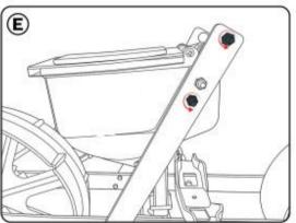
Remove the highlighted nuts from item 4 (main body frame). Remove the same nuts on the reverse side.
