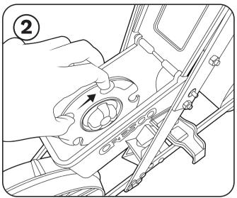
Insert the seed plate into the hopper by placing it over the centre of the mounting and turning the plate clockwise to lock it into position.
