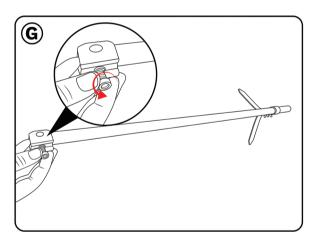
Take item 5 (row marker arm) and remove the nut located at the bottom end.
