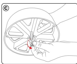
Remove the long bolt located through the middle of item 2 (Rear wheel).
