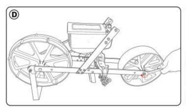
Align the centre hole of item 2 (Rear wheel) to the back hole of item 4 (main body frame). Tighten nut to secure item 2 (Rear wheel).
