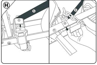
Place the bolt protruding from item 5 (row marker) into the hole shown on item 4 (main body frame). Secure item 5 (row marker) with the nut you removed in step G.
