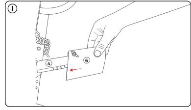
Take item 6 (Depth setting blade) and loosen the wing nut slightly. Slide item 6 (Depth setting blade) onto the depth marker protruding from the bottom of item 4 (main body frame).
