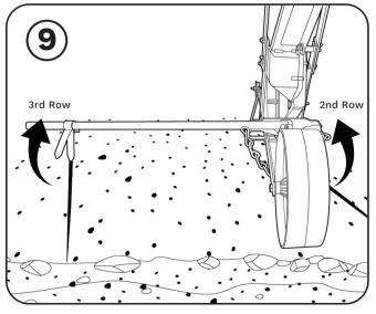
Stop at the end of the first run and place the marker back in its holder in the vertical position. The marker will have left a trail to be followed for the next seeding row (2nd Row). Now place the marker on the opposite side (on your left) and push the seeder along the track made by the marker on your first run (2nd Row).
