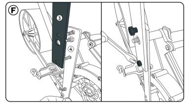
Align the holes of item 3 (Handle Section) with the bolts protruding from item 4 (main body frame). Place item 3 (handle section) onto item 4 (main body frame) and tighten the highlighted nuts.
